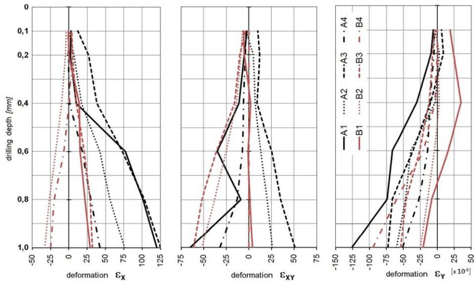
Fig. 5. The strain increments due to welding
