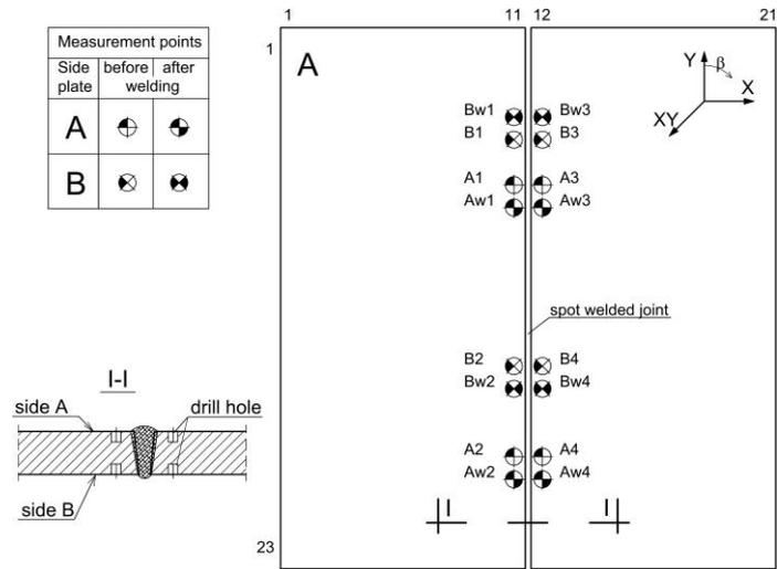
Fig. 1. Geometry of the investigated element
