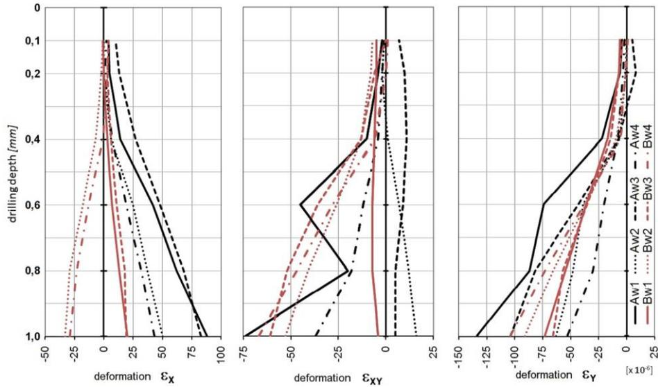
Fig. 4. Strains registered in the experiment, post-welding phase
