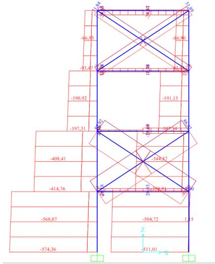
Fig. 7. Envelope diagram of axial forces,  $kN$
