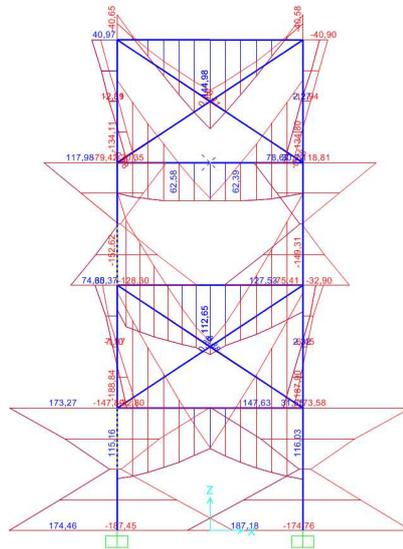
Fig. 6. Envelope diagram of "elastic" bending moments, *kN·m*
