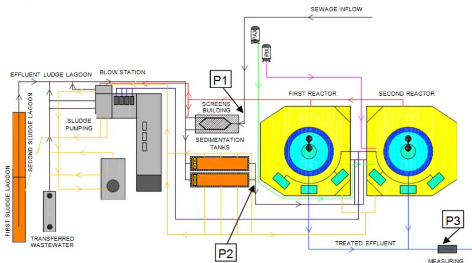
Fig. 2. The technology diagram of the WWTP
